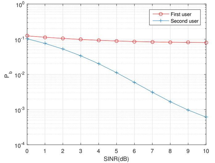
Fig. 4. Each user BER in case of imperfect SIC for fixed power transmission
